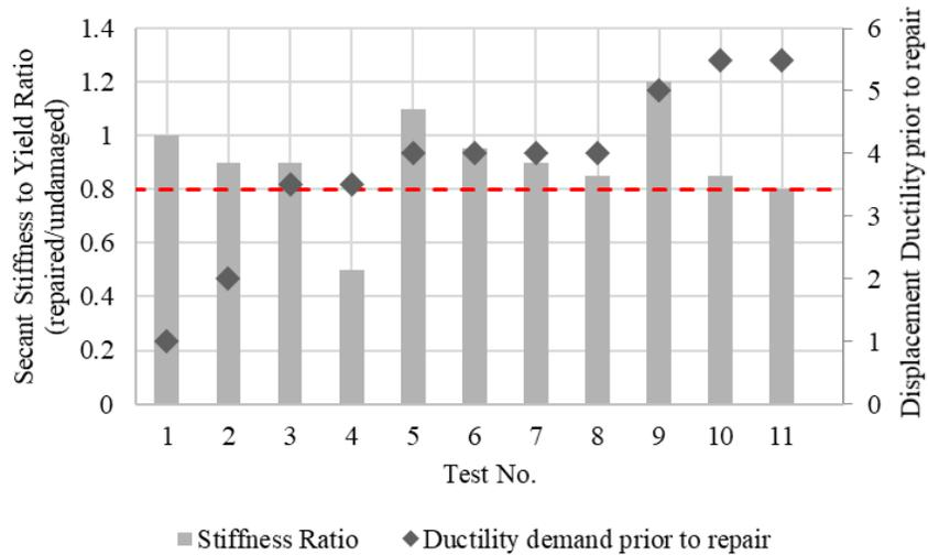
Figure 4. Post-repair secant stiffness to yield ratio vs. maximum displacement ductility prior to repair.
