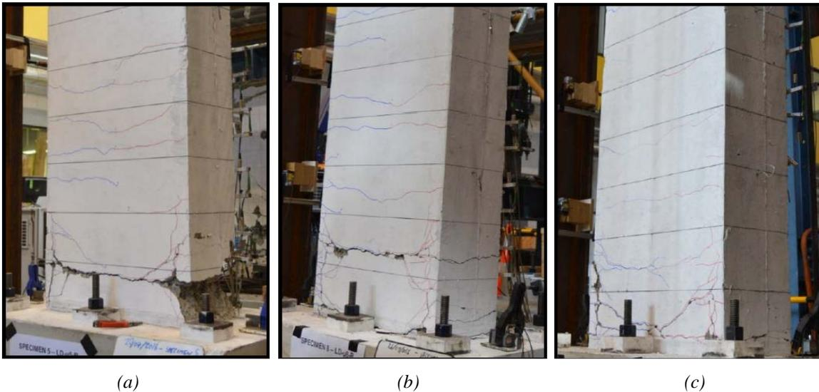
Figure 3. Pre-repair damage state for specimen (a) LD-1-R (b) LD-2-R (c) LD-2-LER-R
