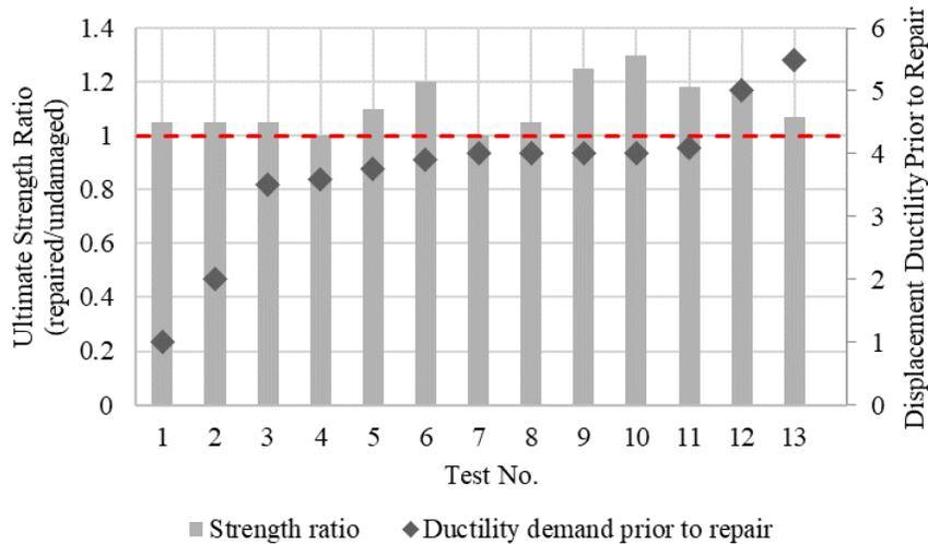
Figure 5. Post-repair ultimate strength ratio vs. maximum displacement ductility prior to repair.
