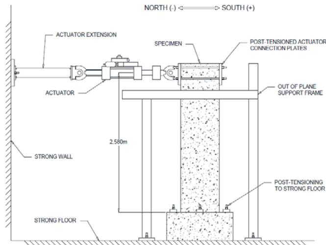
Figure 2. General Test Setup
